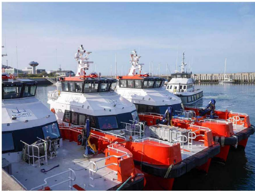
Photo 2. CTVs in the Port of Helgoland (Germany) (photo: Van Oord)
