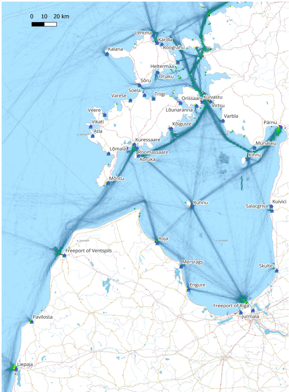
FIGURE 11. THE AVERAGE ANNUAL DENSITY OF YACHTS AND PLEASURE CRAFTS 2017-2023 BY EMODNET. THE MAP IS BASED ON AIS DATA AND SHOWS SHIPPING DENSITY IN 1X1KM CELLS.
