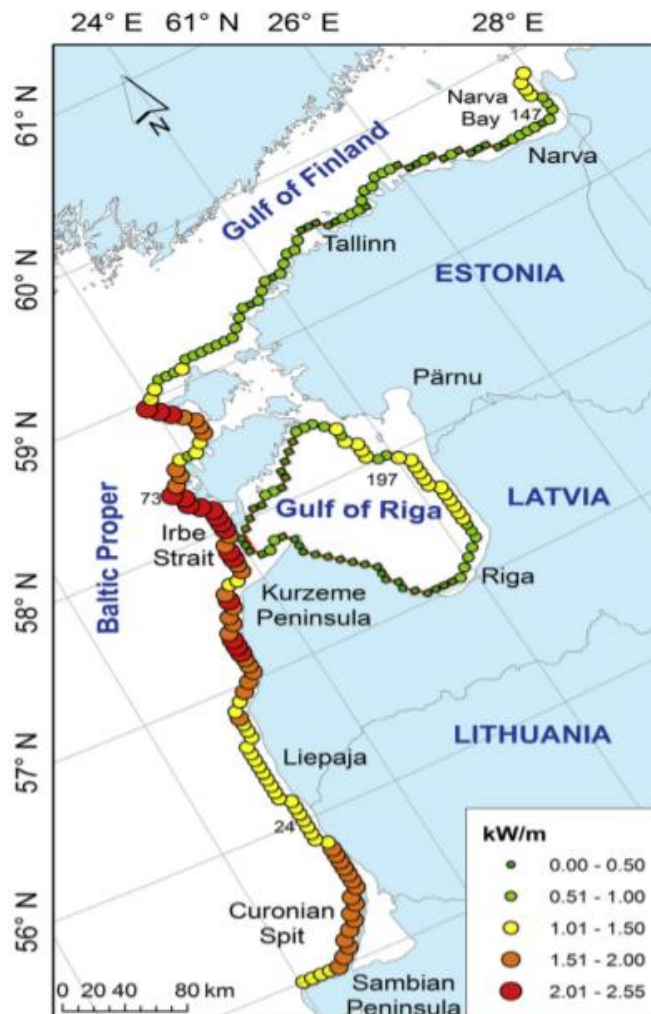
Figure 10.1. Long-term average energy flux along the coasts of the eastern Baltic (146)
